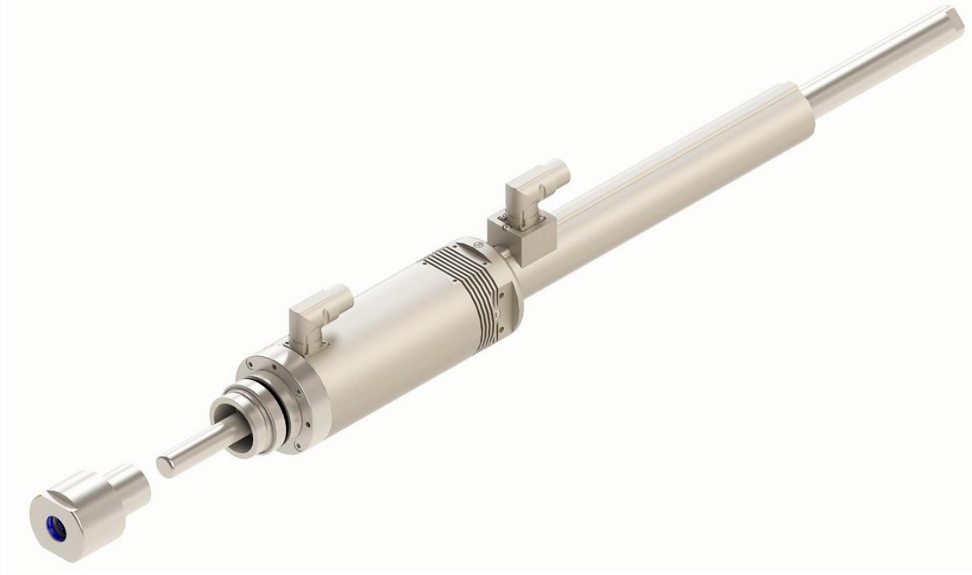
Picture: Front part of the flange, includes sealing and bearings, can be replaced easily. Normally the complete front part with all seals and bearings will be replaced. In case that the seals and bearings are only cleaned the following lubricant has to be used: "fin food Grease 2" from INTERFLON
