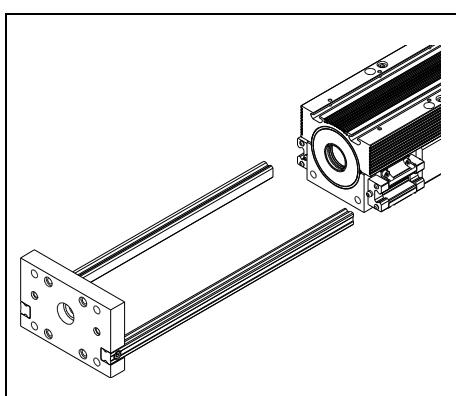
**6. Introduce guide unit carefully without tilting.**
