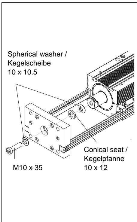
**7. Connect front plate with slider.**
